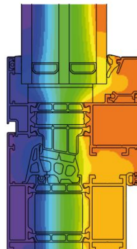
Distribution of isotherms in MB-79N SI window
